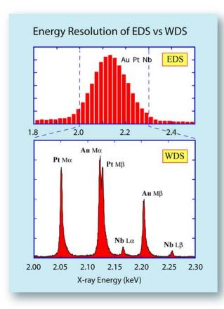
The second major problem with EDS systems is their low count rates and poor reproducibility. Typically a WDS system will have a count rate about 10x that of an EDS system. There are some EDS systems that can collect at a higher count rate, but they sacrifice even more on the energy resolution — their peaks are even wider.
